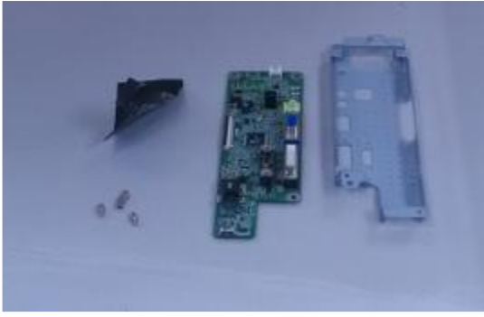
Step.10 Disassemble rear cover assembly
